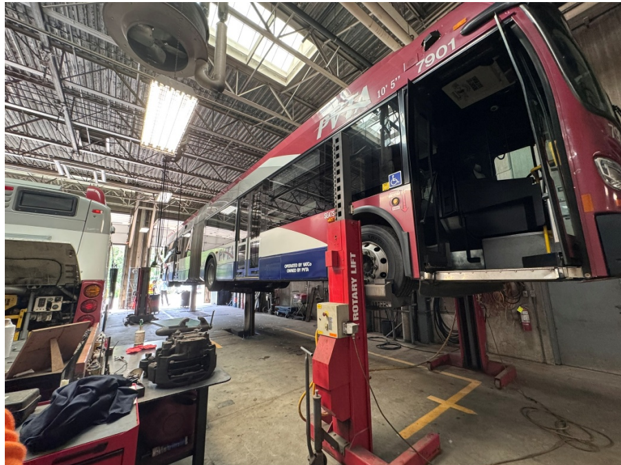
ARCH-09: ARTICULATED BUS LIFTED IN EXISTING BAY
